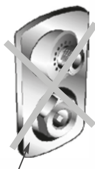
HYDRANT FACEPLATE IN INCORRECT VERTICAL POSITION
