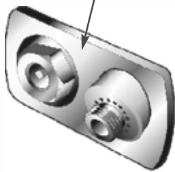
HYDRANT FACEPLATE IN CORRECT HORIZONTAL POSITION
