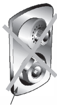
HYDRANT FACEPLATE IN INCORRECT VERTICAL POSITION
