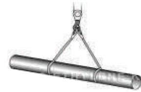
Off-loading on site may be made easier by using skid timbers and strap slings
