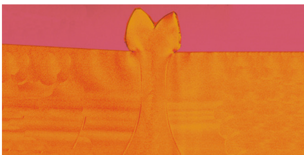
Macro-image of IR (infrared) welding
