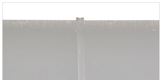
Lateral cut of IR (infrared) welding
